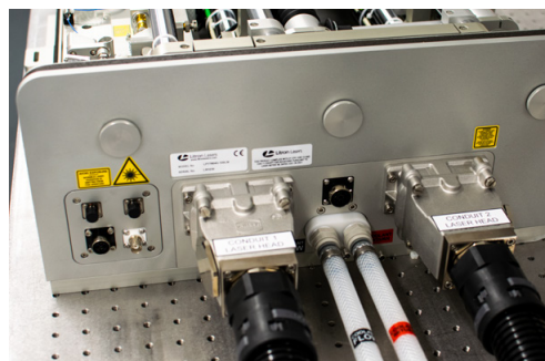
Disconnectable service panel
